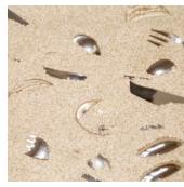
The wet, washed and clean The cutlery rises in a spiral, passing a high-quality warm polishing granulate.
